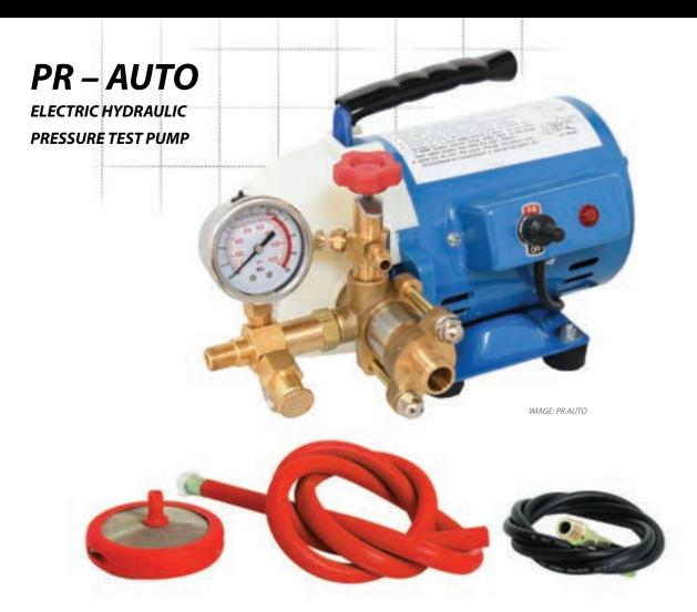
Electric pump designed for pressure testing of system tightness and for filling solar system. The pump's electric motor makes its use exceptionally easy and comfortable. The pump comes with a liquid container, suction hose, high pressure hose, overflow hose and suction filter. Unlike the PR AUTO hand pump, it can also be used to fill the systems with water.
