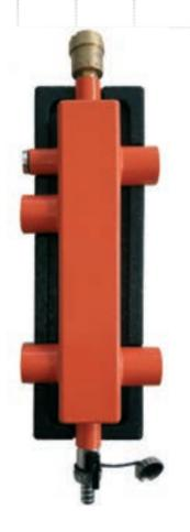
The task of the hydraulic coupling is to separate the boiler circuit from the heating circuit, balance the flows, and keep the pumps running smoothly. Additionally, the coupling protects the boiler against return temperature which is too low.
