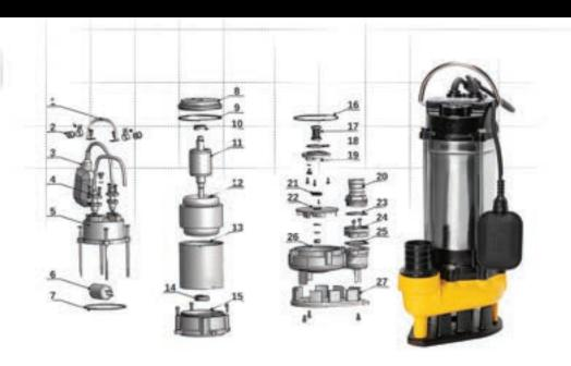
Submersible pumps designed for pumping sewage, dirty water, and water from flooded premises. The pumps are equipped with float switches for automatic pump control. Threaded outlet connection and a set of adapters provide connection of the discharge hose with a hose clamp or fast-connection coupling. WQF pumps are equipped with thermal protection mounted in the motor winding. The motor housing is made of AlSI304 stainless steel, and the impeller is made of grey cast iron.
