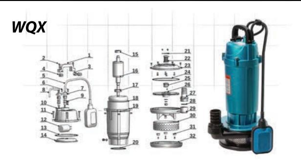
Submersible pumps designed for pumping clean and slightly contaminated water. The motor housing is made of aluminium and the motor is equipped with thermal protection mounted in the winding. High pressure is a special feature of the WQX series pumps. Pump operation is controlled by a float switch. The WQX 250 are available with and without the float switch.
