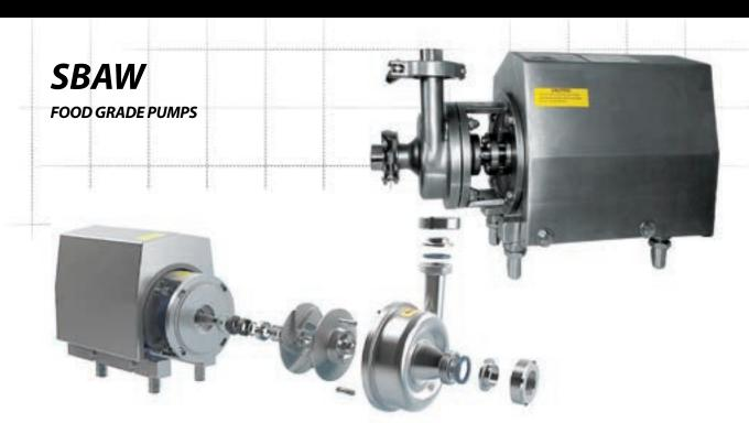
Pumps designed for transporting concentrated or non-concentrated food liquids with up to 50% dry matter content or other food products with a temperature up to 75°C. Centrifugal pumps with open impeller, enclosed motor, and distanced hydraulic body. Inlet/outlet are complete with connections for easy installation. The device has four adjustable legs. SIC/WC (EPDM) mechanical seal. VMQ body seal/
