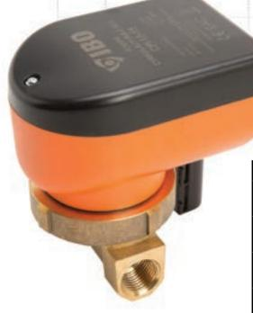
Seal-less circulation pumps designed for forcing hot water circulation. In systems without hot water pumps, after opening the tap, before the hot water starts flowing, cool water remaining in the pipeline will flow first. If a hot water pump is installed, hot water will flow almost immediately after opening the tap. The pump is usually installed upstream the boiler or hot water tank. With years of experience, we have been able to improve previous designs and create the top quality pump.
