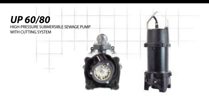
The UP60/80 pumps are equipped with a two-stage hydraulics to increase the maximum pressure. An important feature of KRAKEN 1800 is a multi-channel disk cutting system designed to minimize the risk of clogging. In addition, the outlet is threaded in order to connect a pipeline or fast connection. The pump is supplied with thermal protection mounted in the motor winding.
