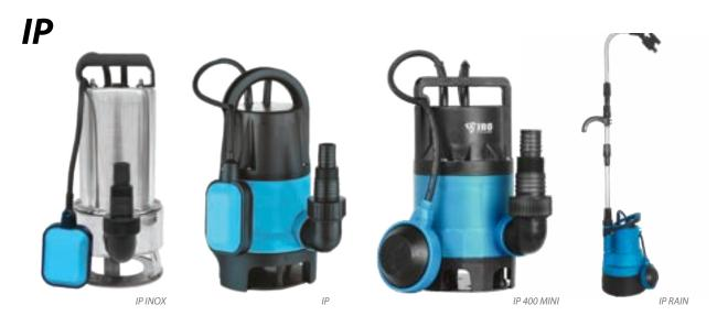
IP submersible plastic pumps designed for pumping clean and slightly contaminated water. The pumps have an outlet connection to which discharge hoses of different diameters can be connected depending on the user's requirements. Small size and light weight make the pumps exceptionally easy to operate and maintain. The pumps are equipped with float switches for automatic pump control. All pumps are supplied with thermal protection mounted in the motor winding.
