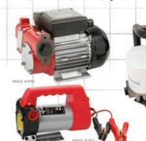
AOPs are displacement vane pumps designed for pumping diesel fuel, heating oil and bio-diesel fuel. The pumps are equipped with thermal protection mounted in the motor winding.
