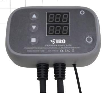
The controller is equipped with 2 LED displays. The current temperature measured by the sensor is displayed as standard on the upper one, while the lower one shows the switch-off temperature. The MENU button toggles the controller into preview mode and switch-on/switch-off temperature settings, as well the anti-stop function setting.
